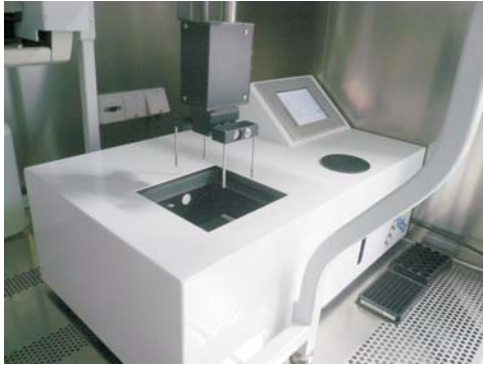
BioLector integrated into a liquid handling system
